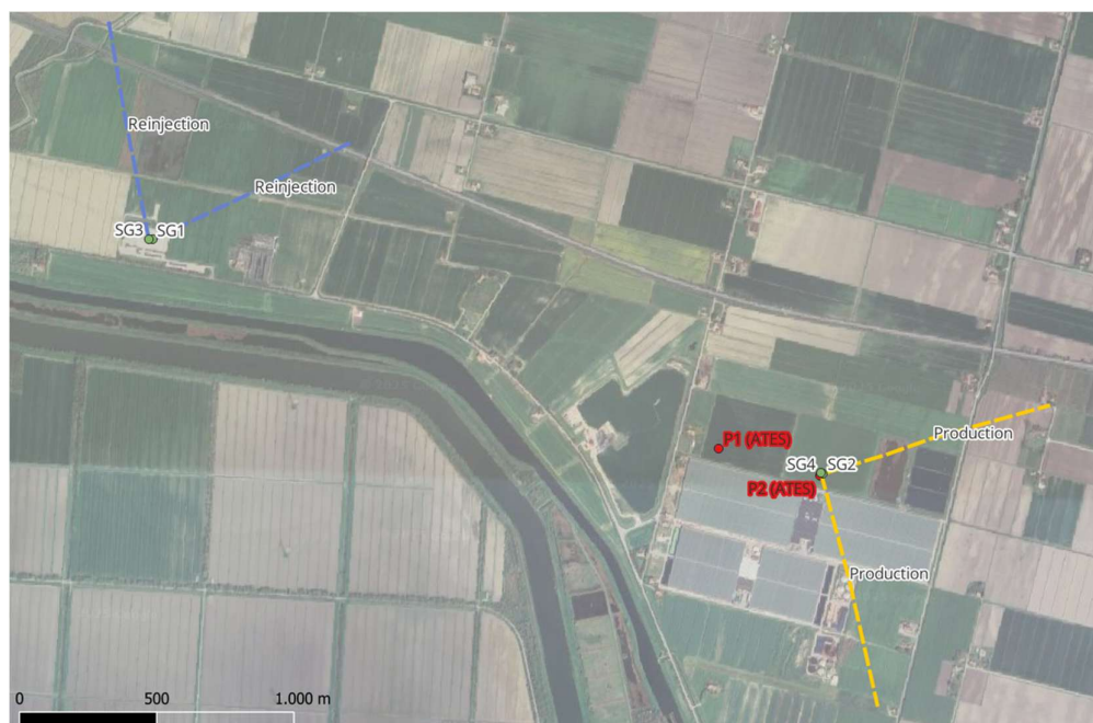
Figure 24 Wellheads and projection of oriented wells (ref. Figure 25). A3-2 reservoir: production (SG2, SG4), reinjection (SG-1, SG-3). Aquifer A1-a: ATES storage (vertical: SG-A, SG-B)
