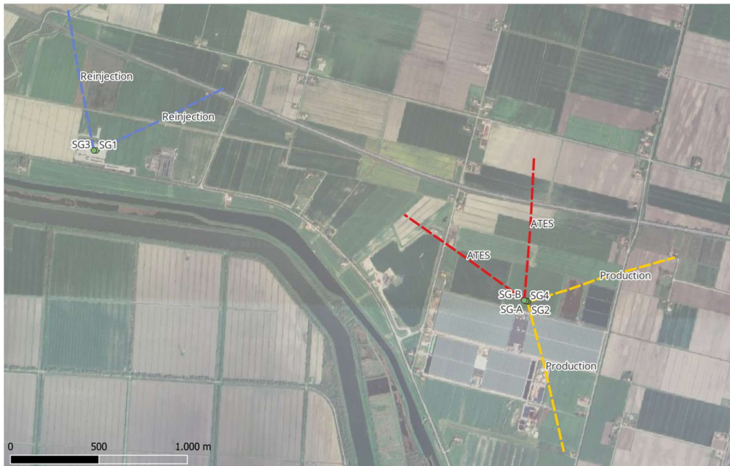
Figure 7 Scenario 1 - Wellheads and projection of oriented wells: production (SG2, SG4). ATES storage (SG-A, SG-B), reinjection (SG-1, SG-3)
